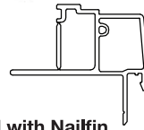
1 1/2" Brickmould with Nailfin
